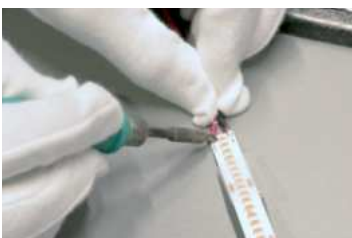
Assembly of LED flex stripes
