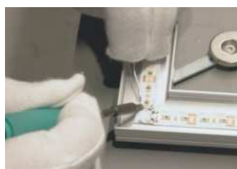
Merging LED flex stripes and aluminum profiles
