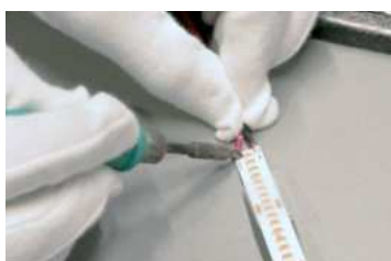
Assembly of LED flex stripes
