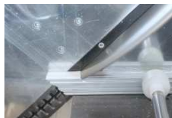
Assembly of LED profiles
