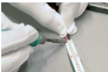
Assembly of LED flex stripes
