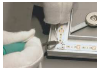
Merging LED flex stripes and aluminum profiles
