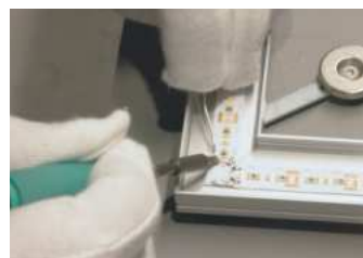
Merging LED flex stripes and aluminum profiles
