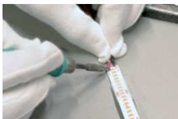
Assemblage de bandes flexibles LED
