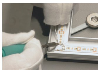
Merging LED flex stripes and aluminum profiles
