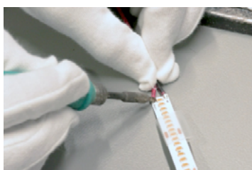
Assembly of LED flex stripes
