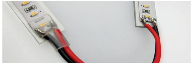
Fig.3 Isolation of solder joints: Preferably with heat shrink tubing Schumpfschlauch
