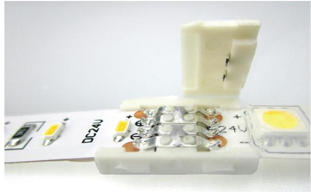
**Hint:** In certain LED Flex strips, the first LED chip is very close to the contact point. To ensure a correct and safe connection, the cap on one side of the clip connector must be removed. The removed cap is shown to the left of the picture. For encapsulated LED Flex strips, remove the casting first with a sharp knife. Otherwise, contacts cannot be connected. The removed casting is shown to the right of the picture.
