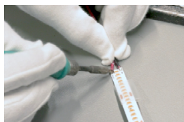
Assemblage de bandes flexibles LED
